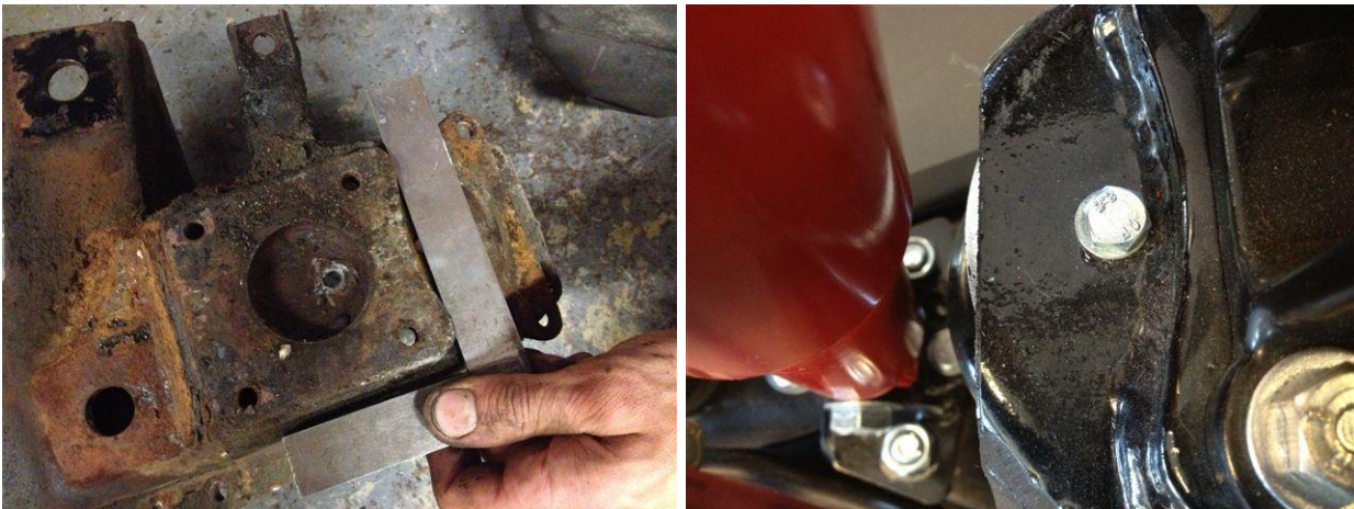
Cross member preparation
